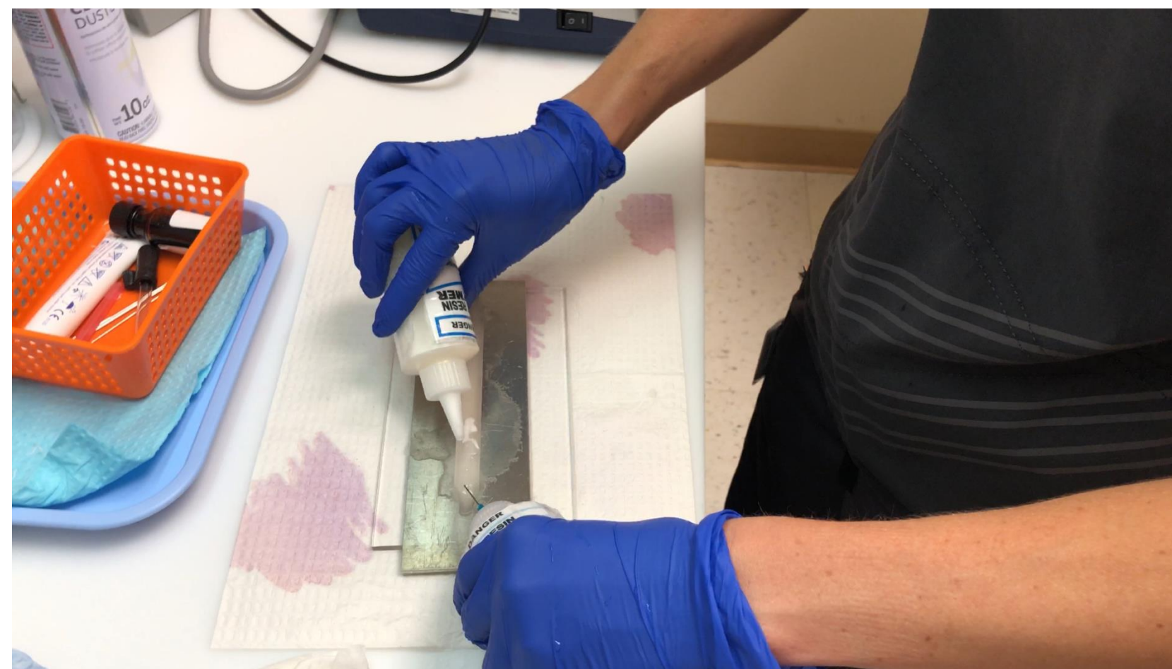
Figure 1: Mold used to cure (and recure) PMMA used for traditional devices
